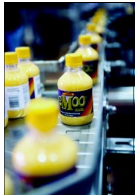
Frank DiMeo/University Photography Bottles of e-Moo are filled in the CU food science department's pilot plant.
